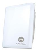
Z500 is an industrial-grade dual-band 2x2 MIMO 802.11ac wireless access point (AP), designed for high user density deployments and backhaul application.
